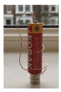
In Science, we have been exploring electricity and have become quite the experts on electromagnetism. This week, we constructed a homopolar motor, which is a direct current electric motor with two magnetic poles , and used this electricity to create motion. We learned that this device is similar to what
